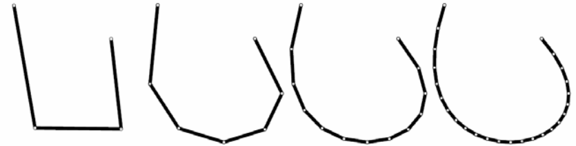
Figure 2.1: Example of subdivision for curves in the plane. On the left 4 points connected with straight line segments. To the right of it a refined version: 3 new points have been inserted “inbetween” the old points and again a piecewise linear curve connecting them is drawn. After two more steps of subdivision the curve starts to become rather smooth.
