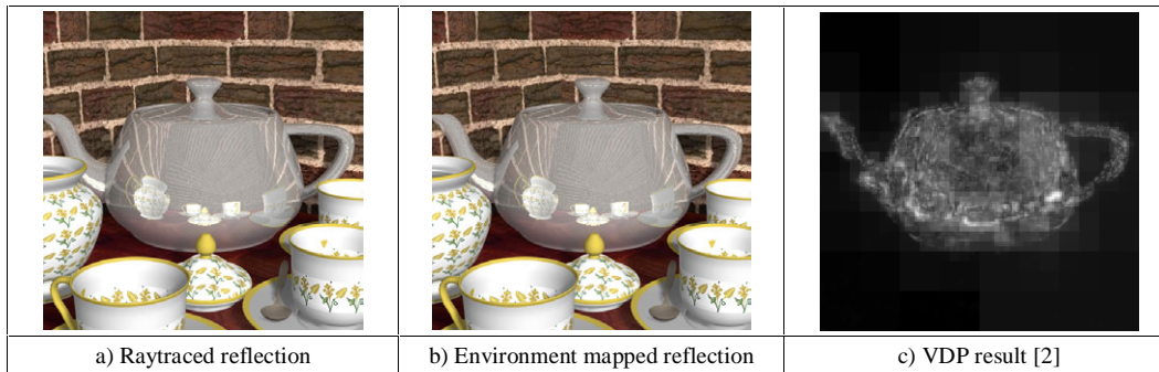
Fig 1. Images rendered with different reflection algorithms and VDP map showing areas of visible difference.
